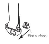
Align the strap hinge to the opposite side of the flat surface of the hook.
