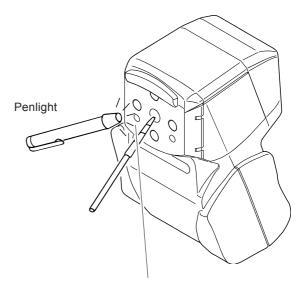
Do not allow the alcohol to contact the sensor window.
