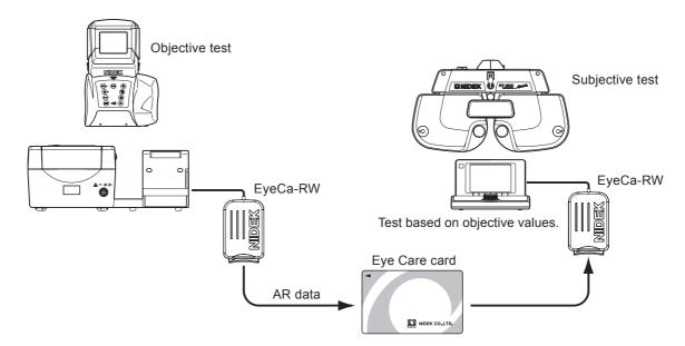
There are two methods to transmit data to the Eye Care card; when measured data is printed and when measured data is not printed.
