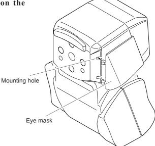
2. Push the hinges into the holes with your thumb.
