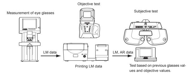
Connect the data input connector (-) on the station to the LM, and connect the data output connector (-) to the RT via the interface cables.
