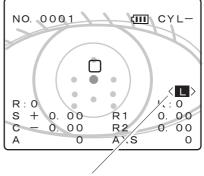
Indication of measuring eye "< >" mark indicates the right eye or left eye has been specified manually.
