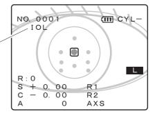
1) Even if abnormal reflected light is detected, the measured results can be obtained by changing its criteria.
